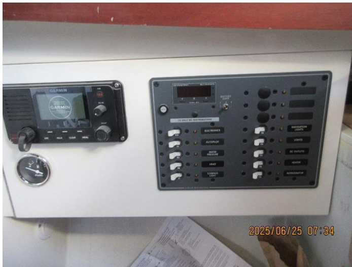
Main D.C. panelboard and VHF radio.
