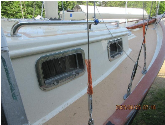
Stbd. side cabin trunk ports and grabrail.
